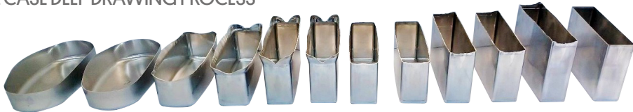
PRISMATIC CELL CASE DEEP DRAWING PROCESS
